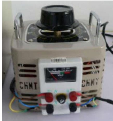
Photo of Voltage Regulator
