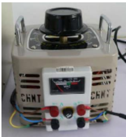
Photo of Voltage Regulator
