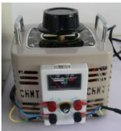
Photo of Voltage Regulator
